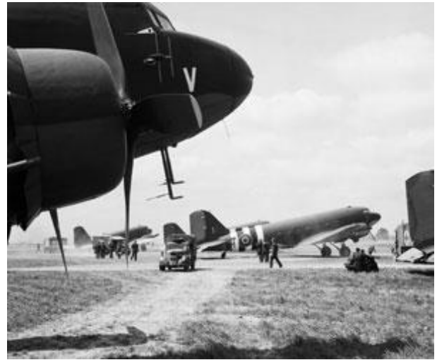
An RAF Dakota with the starboard Rebecca aerial clearly seen just below the cockpit window
